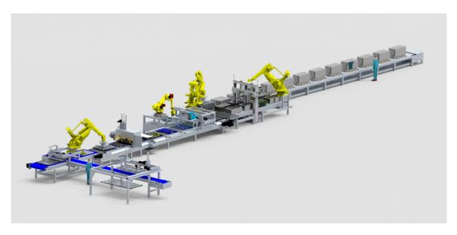
Options for product treatment after curing: shot-blasting, curling, coating, printing. Automatic vertical or horizontal packing on sales pallets.
