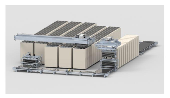
Green slabs on constructed steel pallets with legs. Handling of pallets in and out curing area in different systems (custom made) Shown is system with cranes. Pallet buffering system is opitional.
