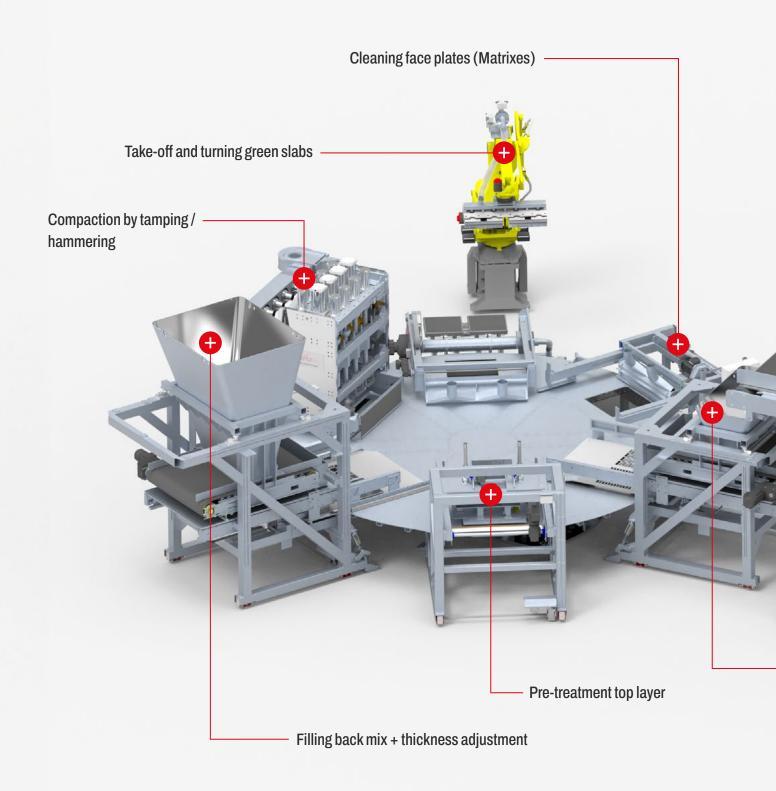
**CYCLE TIMES** 6-10 SECONDS MACHINES WITH 2 OR 4 COMPACTORS
