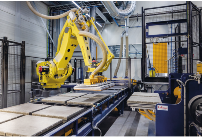
Removing a fresh concrete slab
