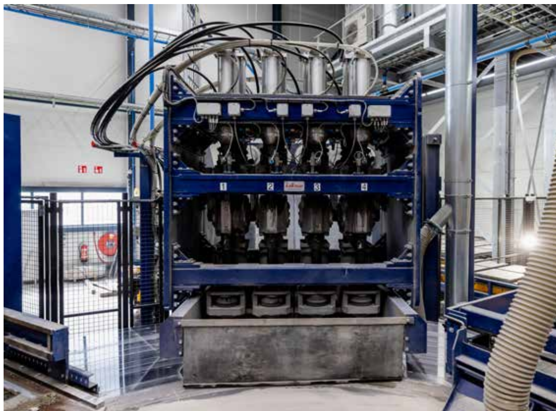
Hammer compaction: Four hammers work together via a control system
